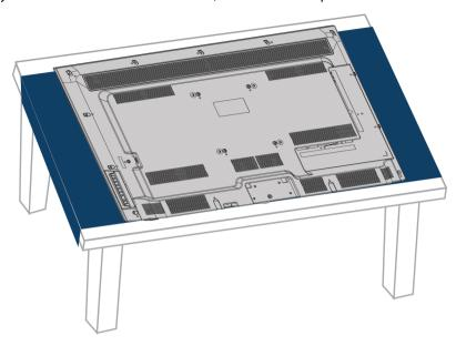
3 Align the screw holes on the stand column with the screw holes on the back of your TV, then secure the stand column to your TV with the four provided  $M5 \times 12$  mm screws (the short screws).
