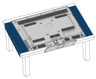
2 If the TV stand is installed, remove the four screws that secure the stand column to your TV.
