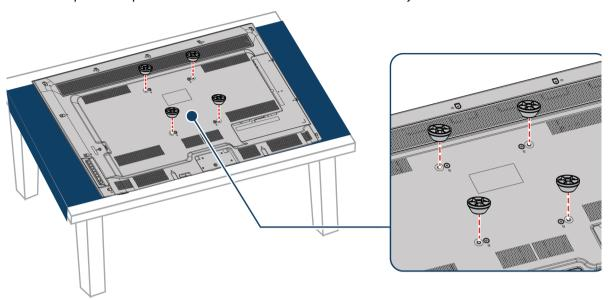
**4** Attach the wall-mount bracket to your TV using either the four provided M6 × 30 mm screws or the screws that came with the wall-mount bracket. See instructions that came with the wall-mount bracket for information about which screws to use and how to correctly hang your TV.
