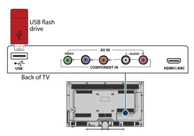
1 Plug a USB flash drive into the **USB** port on the back of your TV.
