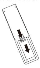
2 Insert two AAA batteries into the battery compartment. Make sure that you match the + and – symbols on the batteries with the + and – symbols in the battery compartment.
